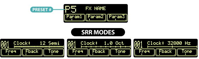
Long press on the encoder knob enter SRR mode, then short click to select from 3 Sample Rate Reduction modes. long press again to exit SRR modes. Default clock is 32.8 kHz.
