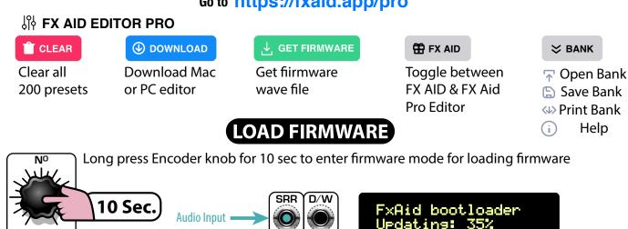
Playback firmware wave file into the SRR input the bar should hover around the middle of the display
